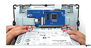
Fix the monitor with the installed daughter PCB to the head unit by using 2 screws at the upper side and 2 screws at the bottom side of the head unit. Page
