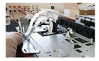
Connect the daughter PCB's ribbon cable "OUT" to the factory monitor board's cable base and connect the factory ribbon cable to the daughter PCB's cable merger "IN".
