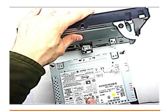
Carefully separate the monitor part from the head unit.
