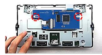
Fix the daughter PCB to the monitor's backside by using the 2 original screws together with the previously fixed spacers.
