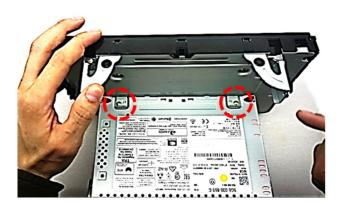
Screw out the two fixing screws at the head unit's upper side.
