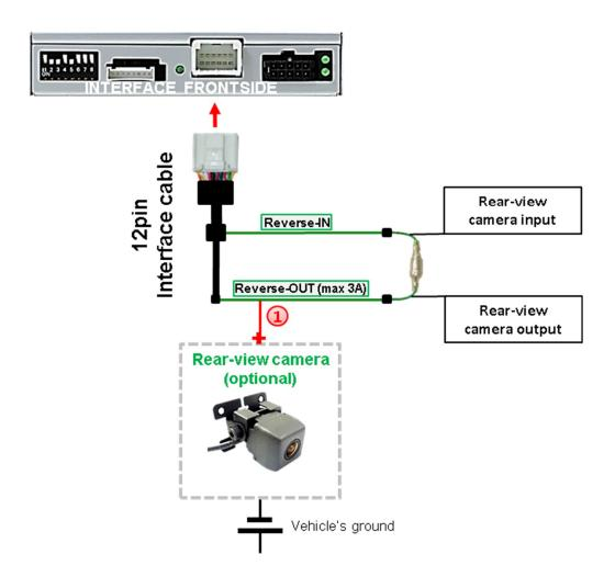
1 The 12 V power supply for the rear-view camera (max 3A) has to be taken from the 12pin interface cabl's green wire "Reverse-OUT" to avoid an unnecessary, permanent power supply to the camera electronic.
