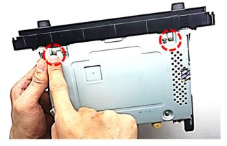
Screw out the two fixing screws at the head unit's bottom side.
