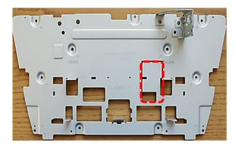
Remove the head unit from the monitor (see VW/Seat). For later leading-out the ribbon cables, cut out the monitor back plate at the marked point and protect the cut edges with fabric tape.
