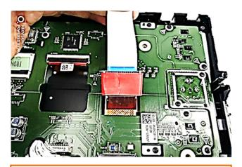
Bevor placing and outleading the daughter PCB's ribbon cables, the ribbon cable merger has to be isolated to save the system from short circuits.
