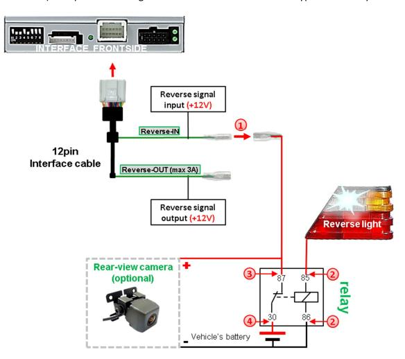
Disconnect the green cable's pre-connected male- and female connectors of the 12pin cable and connect the green input cable "Reverse-IN" to the output connector (87) of the relay.
