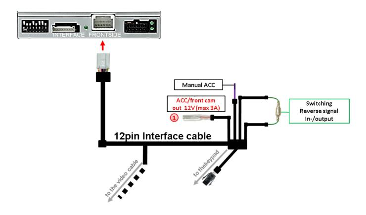
1 The red power supply output ACC/front cam out 12V (max 3A) can be used to power an external source and has a different assignment, depending on the position of dip switch 1 (of 8 dips):
