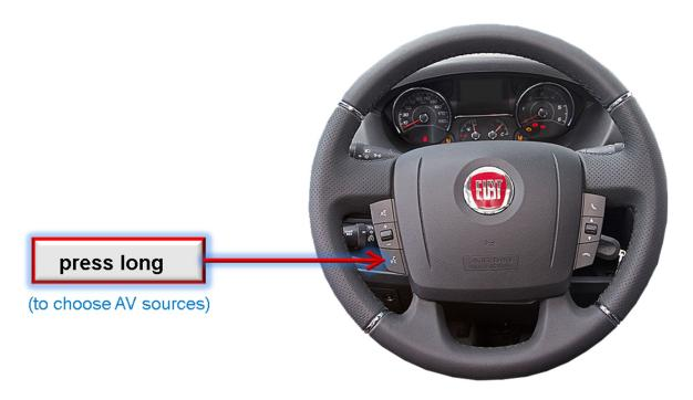
A long press of the steering wheels voice key switches the input from factory mode to the inserted video sources. If, by dip switch setting, all inputs are enabled, the order is the following:
