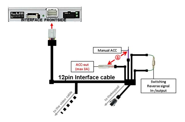
If, after connecting the PNP harness, no interface LED lightens up while the ignition is turned on, the single red wire ACC-out (max 3A) and the purple coloured wire Manual ACC of the 12pin interface cable both have to be connected additionately to S-contact terminal 86s +12V (e.g. glove compartment illumination).
