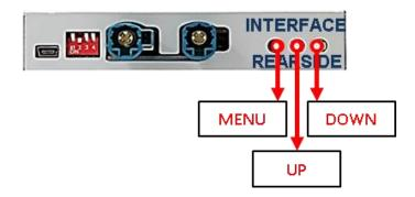
The picture settings are adjustable by the 3 push-buttons on the video-interface. Press the MENU button to open the OSD settings menu or to switch to the next menu item. Press UP and DOWN to change the selected value. The buttons are placed inside in the housing to avoid accidental changes during or after the installation. Picture settings must be done separately for AV1 and AV2 while the corresponding input is selected and visible on the monitor.
