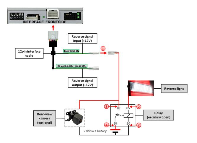
Disconnect the green cable's preconnected male- and female connectors of the 12pin interface cable and connect the green input cable "Reverse-IN" to the output connector (87) of the relay.
