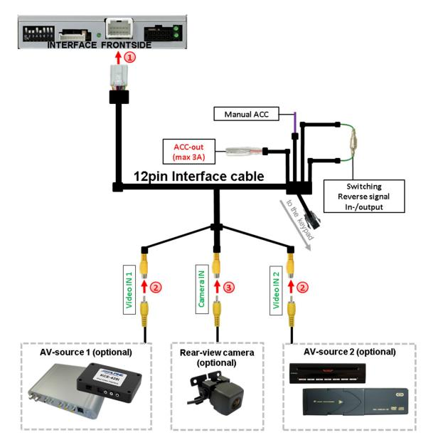
Connect the female 12pin connector of the 12pin interface cable to the male 12pin connector of the video-interface.
