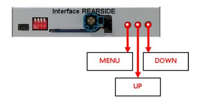
The picture settings are adjustable by the 3 push-buttons on the video-interface. Press the MENU button to open the OSD settings menu or to switch to the next menu item. Press UP and DOWN to change the selected value. The buttons are placed inside in the housing to avoid accidental changes during or after the installation. Picture settings must be done separately for Video1 and Video2 while the corresponding input is selected and visible on the monitor.
