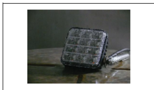
E-R65-1224 after rain test
