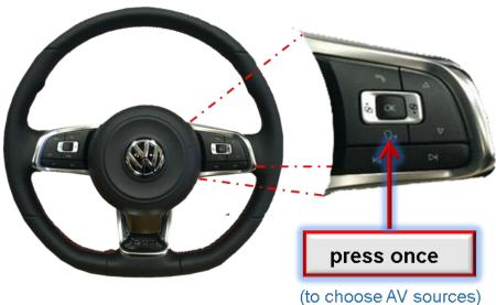
A press of the steering wheels voice key switches the input from factory mode to the inserted video sources. If - by dip switch setting - all inputs are enabled, the order is the following:
