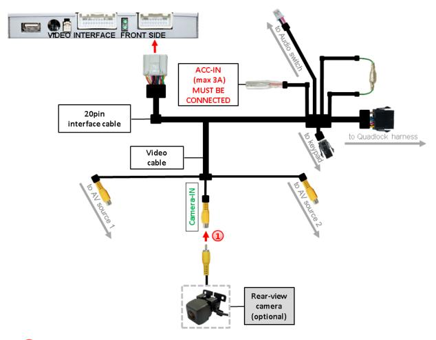
Connect the video-RCA of the after-market rear-view camera to the female RCA port "Camera-IN" of the video-cable.
