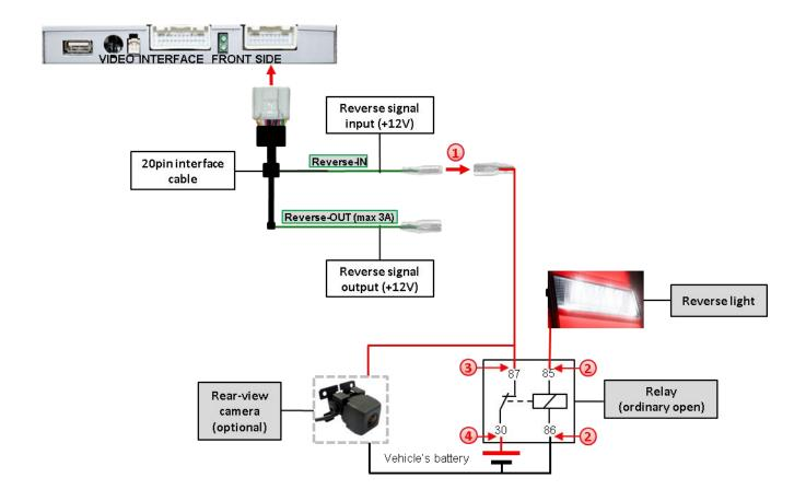
Disconnect the green cable's pre-connected male- and female connectors of the 20pin cable and connect the green input cable "Reverse-IN" to the output connector (87) of the relay.
