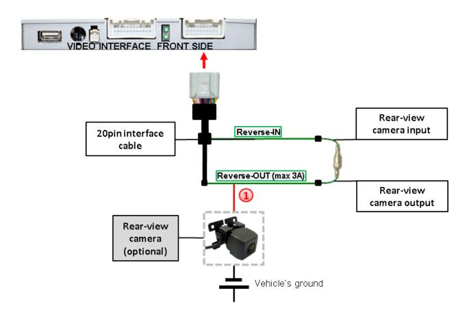
The 12 V power supply for the rear-view camera (max 3A) has to be taken from the green wire "Reverse-OUT" of the 20pin cable to avoid an unnecessary permanent power supply to the camera electronic.
