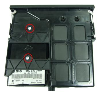
**3.** Remove rubber pocket by pushing out where circled. Lift pocket.
