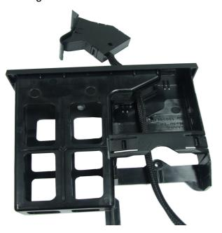
**7.** Re-insert rubber pocket and assemble. Connect USB and 3.5mm jack to aftermarket head unit.
